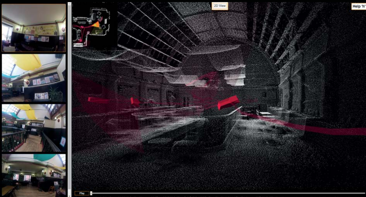
Contextual visual imagery is viewed alongside the 3D point cloud in GeoSLAM Viewer, part of Desktop V3
